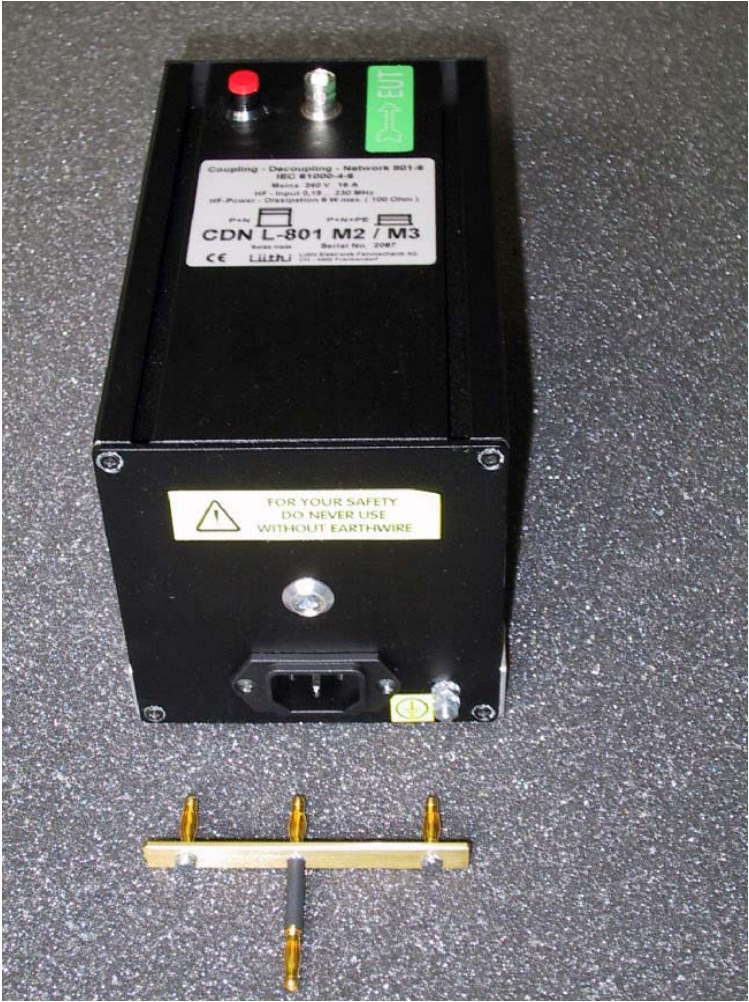
CDN Mains 3 leads, switchable, 4 mm female connectors
