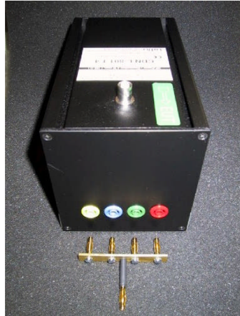
CDN Balanced Lines, 4 mm female connectors
