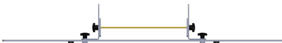
Abb. 3: Line 1 Kalibrierstandard (für hohe Frequenzen) Fig. 3: Line 1 calibration standard (for high frequencies)
